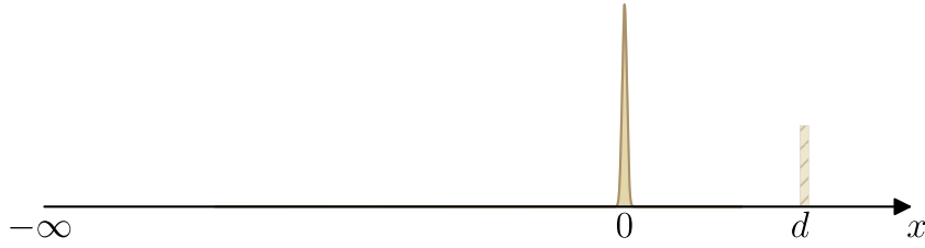
Figure 1. Schematic of our setup. We consider a semi-infinite interval (-\infty, d] . The initial condition is represented by a \delta -distribution located at x(0) = 0 .
