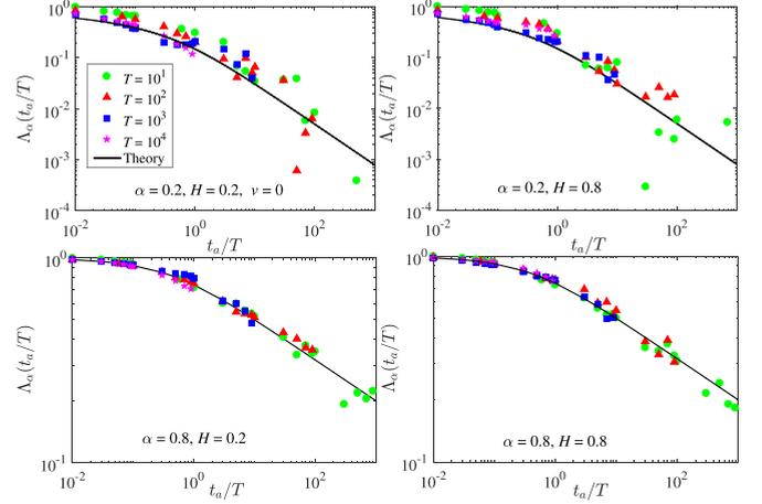
FIG. 6. Aging factor for aged subordinated FBM without drift  $v = 0$  and different measurement times  $T$ . The solid dark curves represent Eq. (20).
