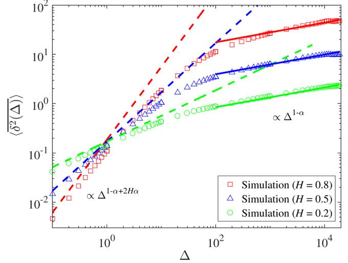
FIG. 8. TAMSD for confined subordinated FBM. The colored dashed curves represent Eq. (12) with  $v = 0$ , the colored solid curves are from Eq. (27). Parameters:  $k = 0.1$ ,  $\alpha = 0.8$ , length of trajectories  $T = 2 \times 10^4$ , elementary time-step  $dt = 0.1$ , and number of trajectories  $n = 300$ .
