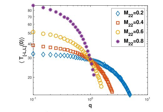
**Figure 14.** Mean first passage time  $\langle T_{[-L,L]}(x_0) \rangle$  versus the ratio *q*. The numerical results are obtained from averaging over  $5 \times 10^4$  realisations on the interval [-L, L] with L = 10. The parameters are  $\boldsymbol{\xi} = (0.5, 0.5)^T$ ,  $v_0 = 2$ ,  $\omega = 1$ , and  $x_0 = 0$ . Moreover we choose  $\phi^{(1)}(\tau)$  and  $\phi^{(1)}(\tau)$  to be power-law PDFs with scaling exponents  $\alpha_1 = 1.5$  and  $\alpha_2 = 1.8$ , respectively.
