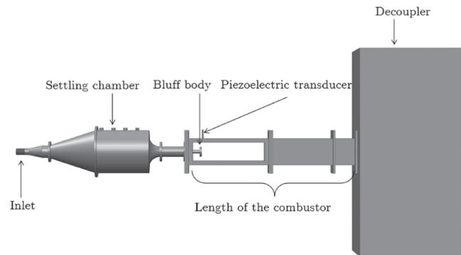
**FIG. 2.** Schematic of the experimental setup. In order to attain different dynamical states, we vary the Reynolds number as a control parameter.
