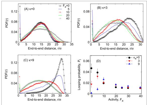
**Figure 2.** Probability distribution of the polymer end-to-end distance for different SPP activities  $F_a$  (denoted by the same colours in panels A, B, C) and varying chain bending stiffness: (A)  $\kappa = 0$ , (B)  $\kappa = 3$ , and (C)  $\kappa = 9$ . In (D) the looping probability  $P_l$  is plotted as function of  $F_a$  for n = 32 and  $\phi = 0.05$ . The error bars for panel D were computed as the standard deviation of the mean values via subdividing the time traces into ten subsets.
