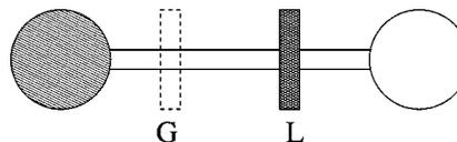
FIG. 1. Schematic picture of a rotaxane switch [1].  $G$  and  $L$  denote the two major stable states of the switching unit (globally and locally stable), a ringlike structure. The two balls at the opposite ends of the main dumbbell-like molecule strand are stoppers.
