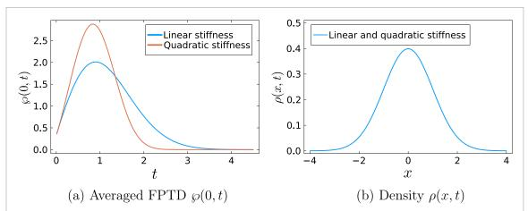
**Figure 3.** (a) Comparison of the FPTD averaged over initial positions for two different choices of the stiffness protocol  $\kappa(t)$ . For the blue curve we used the linear function  $\kappa(t) = T(t) = 0.1 + t$ , while for the orange curve we used the quadratic form  $\kappa(t) = T(t) = 0.1 + t + t^2$ . In both cases we use  $\gamma = 1$ . (b) Density  $\rho(x,t)$ , which is equal for the two cases of linear and quadratic stiffness
