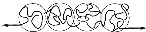
FIG. 5. Qualitative representation of a stretched polymer with a SL. The loop created by the SL is contained within a single blob, and its size is determined only by the number of the monomers in the blob.
