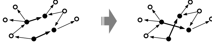
Fig. 3.13 Generating random networks with preserved degree distribution: At each iteration, two edges ( a \rightarrow b ) and ( c \rightarrow d ) are selected at random and rewired as ( a \rightarrow d ) and ( c \rightarrow b ), provided that the respective edges do not already exist. Note that for undirected networks, there are two possible ways to rewire the links.
