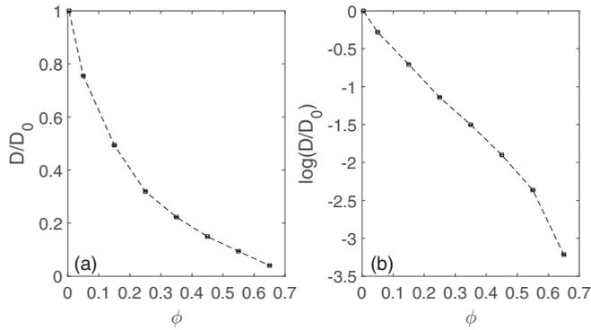
FIG. 15. (a) Translational diffusivity as a function of  $\phi$  obtained via Eq. (18) from the MSD of diffusion of single, nonconnected monomers. (b) Linear-log<sub>e</sub> plot of the data of panel (a). Parameters are the same as in Fig. 2.
