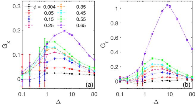
FIG. 6. Non-Gaussianity parameter (22) for (a) translational and (b) rotational motion of the dumbbells plotted against the lag time  $\Delta$  for a set of varying  $\phi$  (see the legend). The lines connecting the points guide the eye. Note that panels (a) and (b) have different vertical scales.
