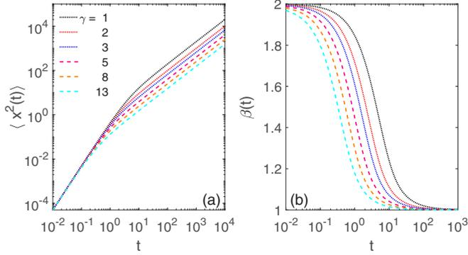
FIG. 11. (a) Translational MSD for the COM motion of a *single* dimer governed by Eq. (4) (see also Eq. (17) in Ref. [140]) for varying friction coefficient  $\gamma$ , with  $k_B\mathcal{T} = 1$  and  $m = 1$ . (b) MSD scaling exponent for the simulation data of panel (a), calculated via Eq. (17).
