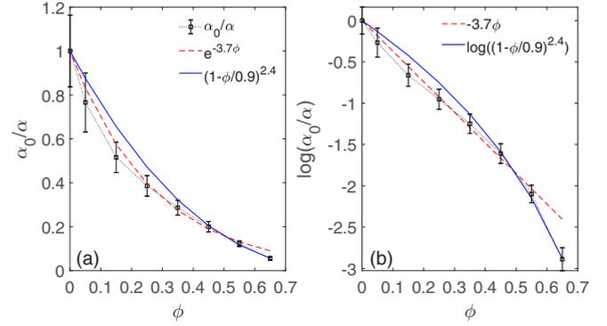
FIG. 10. Normalized inverse decay constant of  $C_d^{\text{env}}(\tau)$  given by  $\alpha_0/\alpha$  from Eq. (25) shown as function of crowding fraction  $\phi$  in linear (a) and  $\log_e$  (b) scale. The fit functions used are listed in the legends. Here,  $\alpha_0 = \alpha(\phi = 0.004)$  and the error bars are indicated.
