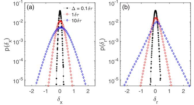
FIG. 5. (a) Translational and (b) rotational displacement-PDFs for the highest crowding fraction  $\phi = 0.65$ , computed for several values of the lag time  $\Delta$  (see the legend) and for other parameters (such as  $m$ ,  $\gamma$ ,  $\tau_0$ ,  $\epsilon$ , and  $T$ ) as in Fig. 2.
