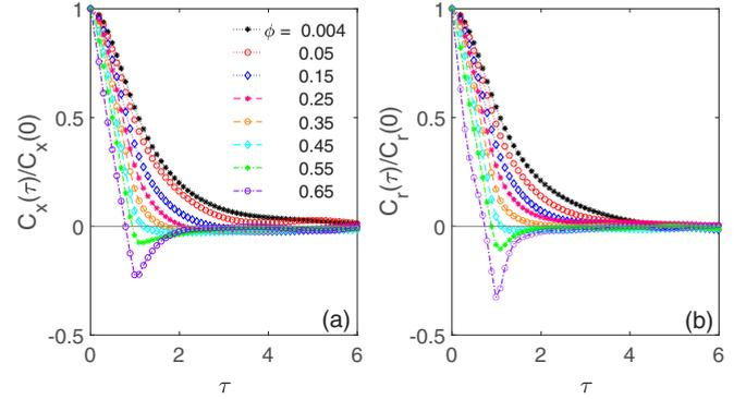
FIG. 7. Normalized (a) translational and (b) rotational displacement-ACFs as a function of the correlation time  $\tau$  computed for varying crowding fractions  $\phi$  (see the legend). The presented ACFs are normalized to the respective initial values at  $\tau = 0$ . Parameters: the lag time in Eq. (24) is  $\Delta = 1 \times \delta\tau$ .
