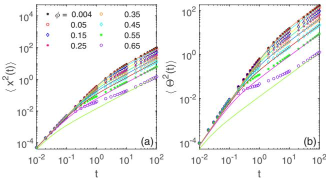
FIG. 12. (a) Translational and (b) rotational MSD for diffusion of dimers at different crowding fractions  $\phi$  (see the legend, symbols), plotted for  $\gamma = 1$  for the TAMSD data of Fig. 2, with the analytical result Eq. (16) shown as the solid curves.
