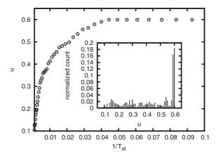
**Figure 3.** Plot of the SA estimate of the statistical weight factor u versus the annealing temperature  $1/T_{\rm at}$ . Inset: histogram showing the Metropolis sampling of instantaneous fluctuations in u for the entire range of annealing temperature performed during the optimization process. The main figure plots the best u at a given temperature step obtained from the fluctuating data shown in the histogram.
