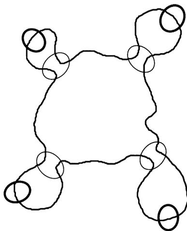
Fig. 2. Central ring polymer from which a number of slip-links separate off fringe loops. Within the latter, sliding rings are placed. If the sliding rings are immobile, the central loop is the overall governing structure. If the sliding rings are activated and become mobile, the fringe loops tend to be large, which leads to a decrease of the mean extension of the compound.
