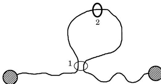
Fig. 1. Linear polymer chain with stoppers at both ends. A permanent loop is formed by the slip-link, 1, holding two parts of the chain close together. On the loop, a sliding ring, 2, is placed.
