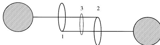
Fig. 4. 'Molecular muscle' consisting of two interlocked rings 1 and 2 with attached rod-like molecules. Within this structure, sliding rings, 3, can be placed, which, if activated, tend to contract the muscle by entropic forces.
