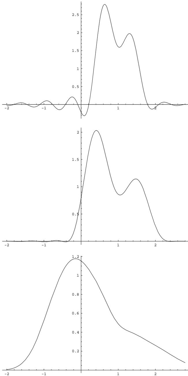
Fig. 2. Temporal evolution of the propagator  $W(x,t)$  of the enhanced fractional Ornstein–Uhlenbeck process. The counter-motion of the two asymmetric humps, and the simultaneous depletion of the initial value region  $x_0 = 1$  are distinct. The number of summation terms is 80. The plots correspond to the dimensionless times 0.2, 0.4, and 1.2. Eventually, the stationary symmetric Gaussian PDF is reached.
