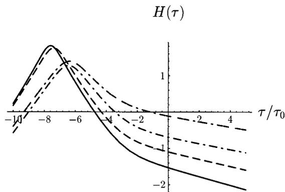
FIG. 7. Relaxation time spectrum for NR32237. Filler content: 0,30,60% phr. The higher the filler content the more the power law tail is shifted to higher vertical values.
