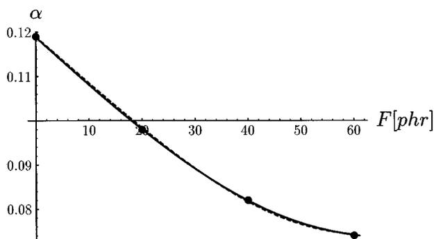
FIG. 12. Difference of the fractal parameters  $\alpha = q - \mu$  for the series S10. Fit by modified VTF law for  $F_{\text{crit}} = 0.901$  phr and  $0.805$  phr (dashed).
