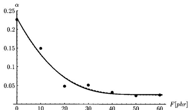
FIG. 11. Difference of the fractal parameters  $\alpha = q - \mu$  for the series NR32237 fitted by modified VTF law for  $F_{\text{crit}} = 0.936$  phr and 0.798 phr (dashed).
