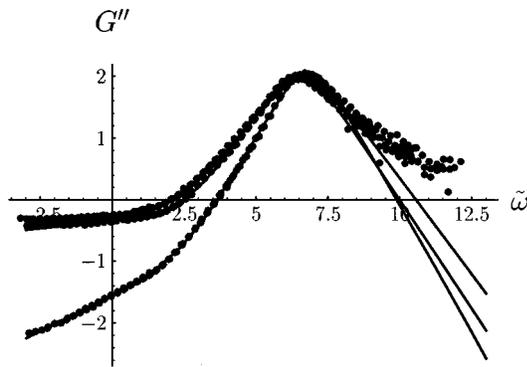
FIG. 6. Loss modulus for NR32237 with a varying filler content  $F=0,20,40\%$  phr (from bottom to top curve).
