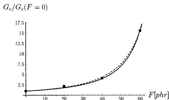
FIG. 10. Normalized equilibrium modulus vs filler content for the series S10.
