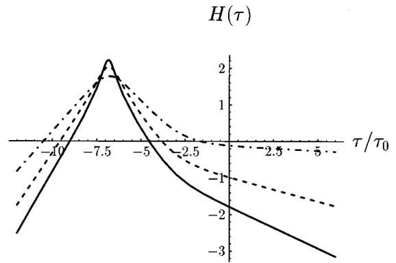
FIG. 8. Relaxation time spectrum for S10. Filler content: 0,20,40,60% phr. The higher the filler content the more the power law tail is shifted to higher vertical values.
