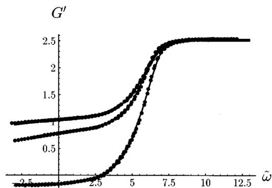
FIG. 5. Storage modulus for NR32237 with a varying filler content  $F=0, 20, 40\%$  phr (from bottom to top curve).
