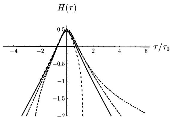
FIG. 3. Spectrum  $H(\tau)$  for  $G_m=9$ ,  $G_e=1$ , and the fractional parameters  $q=0.7$  and  $\mu=0.3, 0.5, 0.7, 0.9$  (from right top to bottom). The full line corresponds to  $q=\mu$ .
